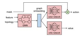
Figure 6: Actor and Critic network architecture of Neuro-Plan.
