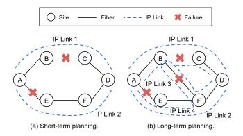
Figure 1: An example for network planning to satisfy a 100Gbps flow from A to D under any of the three single-fiber failures. (a) Short-term planning uses two IP links A-B-C-D and A-E-F-D. (b) Long-term planning adds a new fiber B-F, and uses two IP links A-B-C-D and A-B-F-D. Other options (e.g., using A-E-F-D and A-E-F-B-C-D) consume more fibers.
