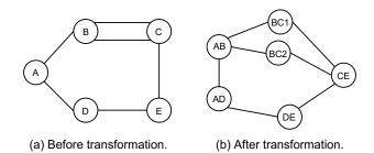
Figure 5: Node-link transformation can handle parallel links. The node names show the corresponding relationship between nodes and links.
